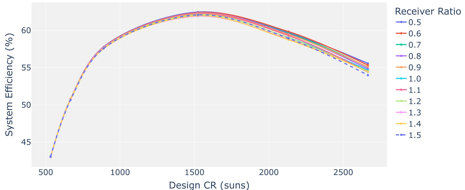
Impact of Varying Heliostat/Receiver Ratio on System Efficiency - 1200 °C 20 MW
